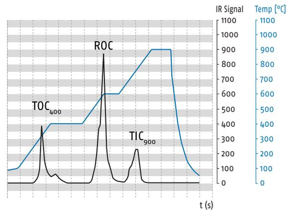
Figure 1. Three-step temperature program of the soli TOC cube using a Cambisol B Horizon soil sample.
