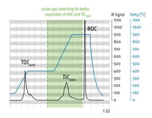
Figure 2. Two-step temperature program with gas switching of the soli TOC cube using a Cambisol B Horizon soil sample.
