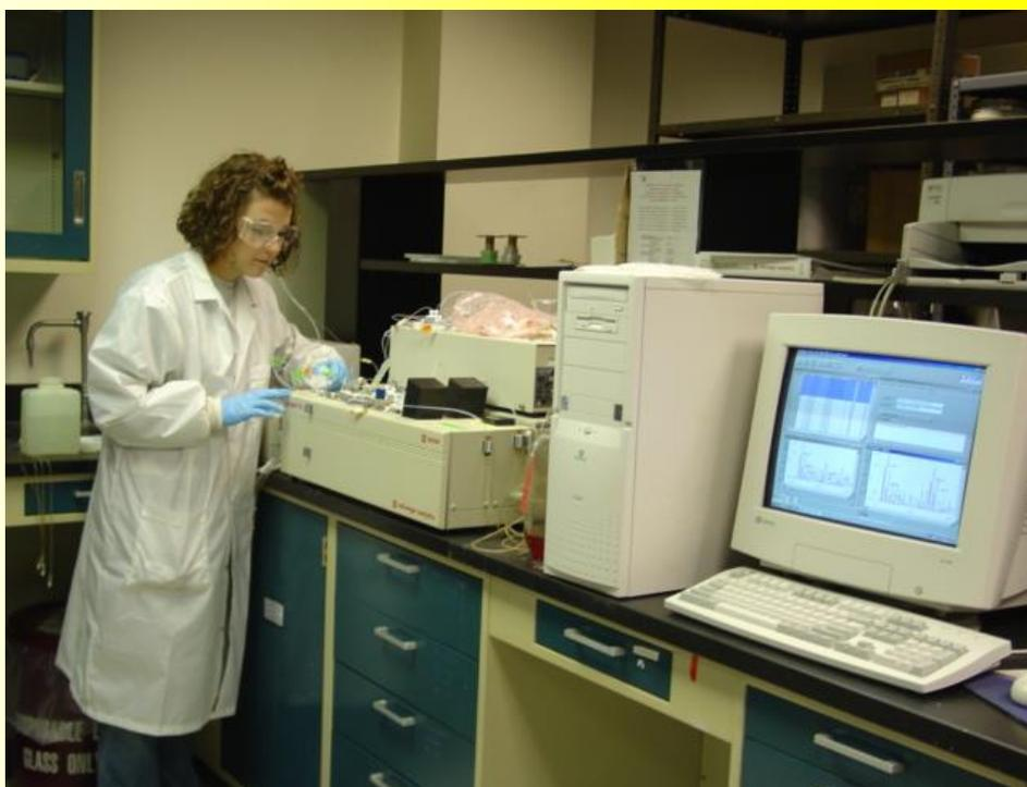
• **Instrument:** Shimadzu SSM-5000A and TOC-5000A Analyzer
