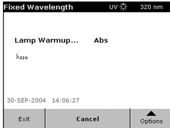
**NOTE** For the most accurate and stable measurements in the UV range, let the lamp warm up for five minutes before taking the first reading.
