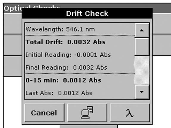
The screen displays the last reading and slope for each 15 minute interval. At the end of the hour, the instrument calculates and displays the overall values.
