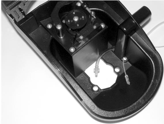
**3** Turn the Sipper Module on its side.
