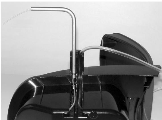
**5** Hold the rubber fitting with the ridges over the grooves and push it firmly onto the guide tube and the waste tube.
