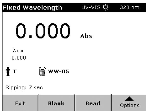
Leave the inlet tube in the blank solution or the sample vessel until the Sipper pump stops and the settling cycle begins.
