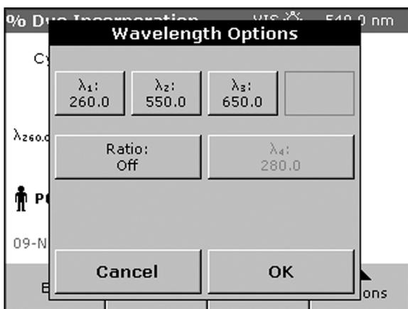
Touch  $\lambda_1$  to  $\lambda_3$  to change the default wavelengths settings and enter the desired wavelength using the numeric keypad.
