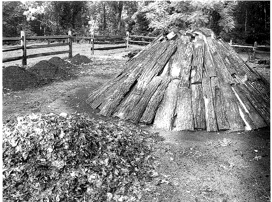
Charcoal pits usually had three tiers and might contain 25 to 50 cords of wood. The demonstration pit at Hopewell is smaller at about 5 to 6 cords. Note the piles of leaves and charcoal dust ready to cover the pit.
