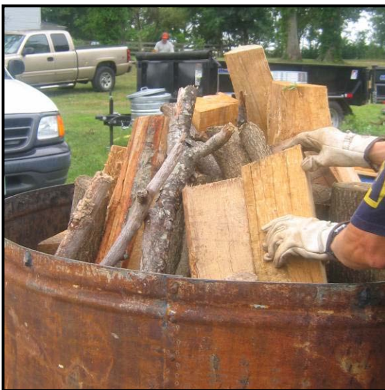
These images show a “New Hampshire” style kiln being loaded
