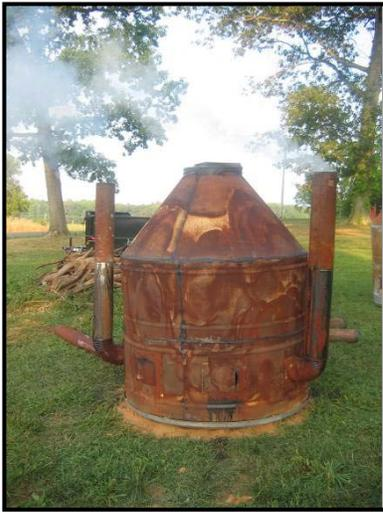
**The charcoal-making process:** A fire is started in the center of the kiln, using the “core” of dry kindling wood. Once a fire is started, chimney stacks are added, and the ventilation ports are closed to limit the flow of oxygen. The oxygen-poor environment allows the wood to “cook” into charcoal, but prevents the full combustion of the wood. Within 10-20 hours, the water, hydrogen, methane, volatile compounds, and tars burn off, and the wood is converted into charcoal.
