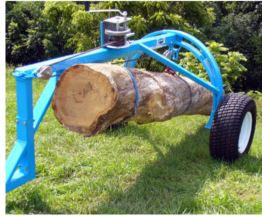
Figure 8. A log arch, fetching arch or sulky lifts the end of the log being dragged to keep it from digging into the earth, rocks, roots, or stumps.
