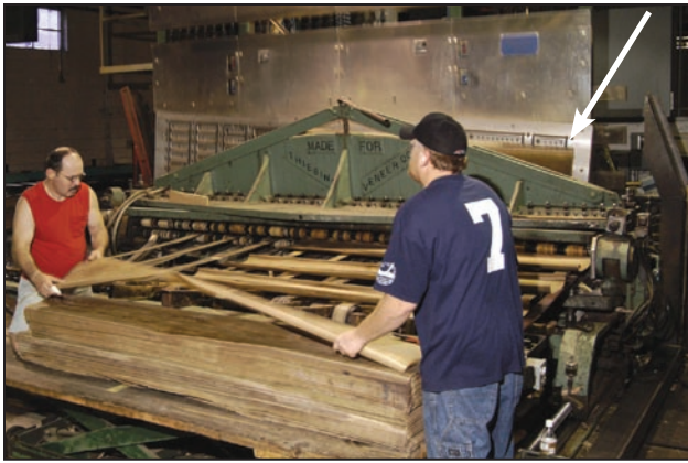
Figure 1. Veneer slicing operation showing the flitch or log half (back and right) being moved up and down against a stationary knife and the individual veneer sheets being stacked in the order that they are sliced.
