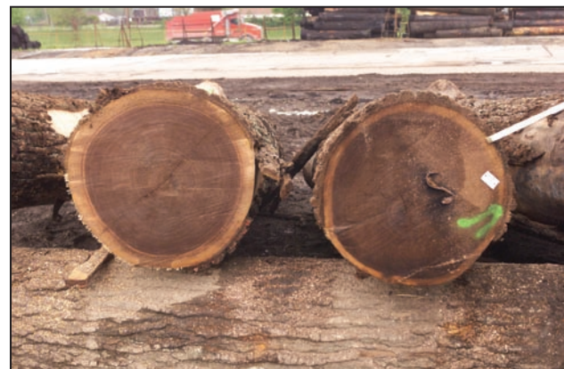
Figure 9. Fast growth trees tend to have a wide sapwood (left); slow growth trees tend to have a narrow sapwood (right).
