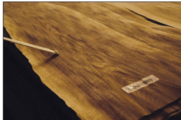
Figure 3. Buckle or irregular surface in walnut veneer. Note the irregular appearance of the tag.
