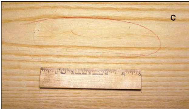
Figures 22A, B, C. The zigzag line on the debarked surface of this ash log is called glassworm, and it results in a similar distortion in the veneer. Another pattern called turkey tracks is shown in the second veneer sample.
