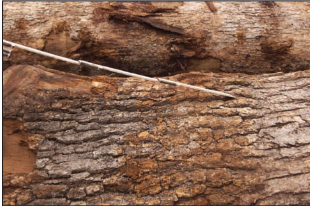
Figure 16. Bulge at the base of some large white oak, also called “soda bottle effect” are not considered defects.
