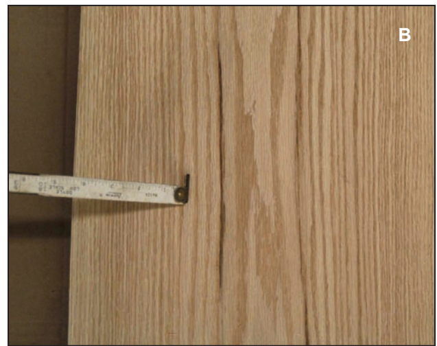
Figures 12A, B. Mineral stain following a growth ring on the end of a white oak log and appearance of mineral stain in white oak veneer.
