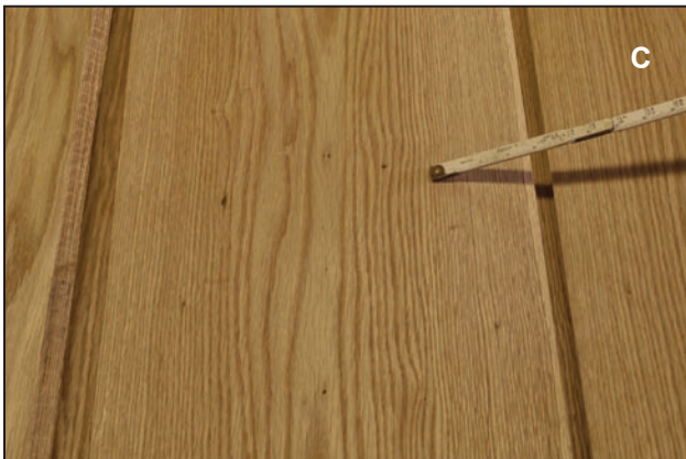
Figures 13A, B, C. Pin knots in the bark and log surface of a white oak log as well as in the oak veneer.
