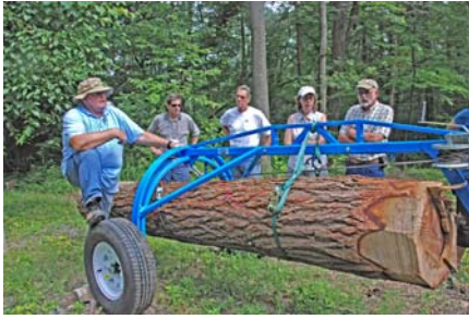
Lee Stover demonstrates a tractor-driven log arch as part of the woods safety presentation.
