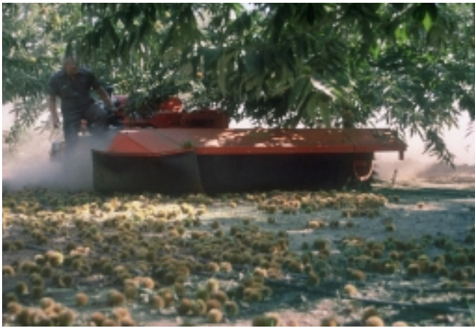
Figure 13. A chestnut sweeper moving nuts into a windrow.
