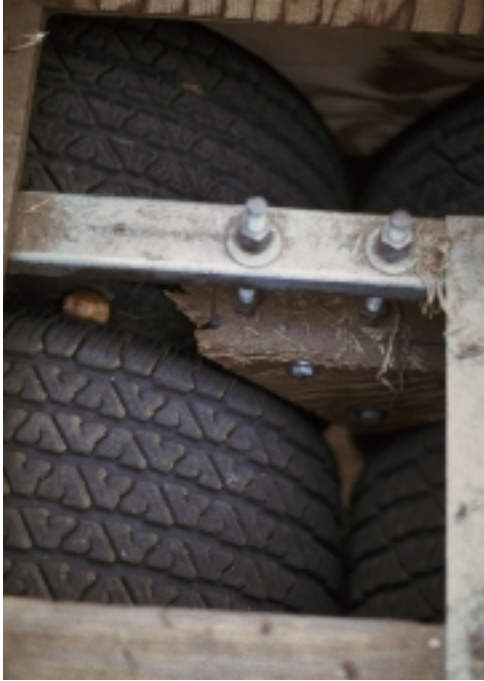
Figure 16. A chestnut wringer, made from tires, can be used to remove nuts from the burrs.
