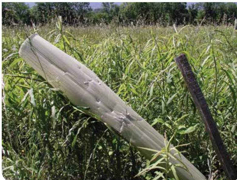
FIGURE 21 TOP RIGHT Rodent gnawing damage. D. JACKSON PENN STATE EXTENSION
