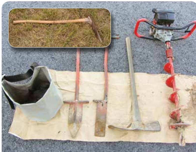
FIGURE 16 TOP Some common tree planting tools include a tree planting bag, KBC bar, dibble bar, mattock, and auger. An auger works well for planting hardwood seedlings with relatively large root systems. A hoedad (inset), similar to a mattock, is another tree planting tool commonly used when planting large quantities of conifers. D. JACKSON PENN STATE EXTENSION
