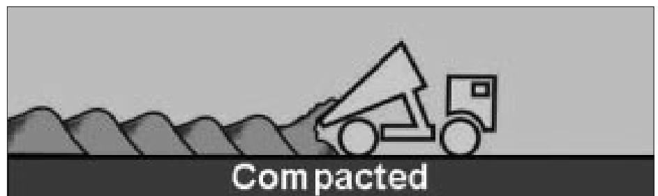
Cartoon depicting the concept of applying loose dumps of soil over compacted, strip mined land.
