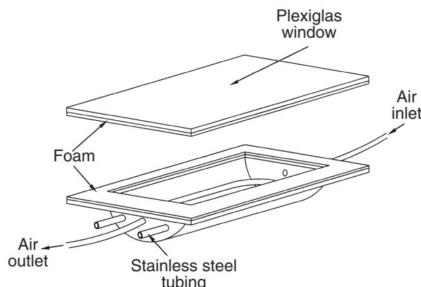
**Figure 1.** Schematic illustration of a chamber for measuring respiration on intact single-root branches. The lid of the chamber is 8.5 cm wide by 11.5 cm long. Water from a heated/refrigerated water bath is circulating through the stainless-steel tubing to control chamber temperature.
