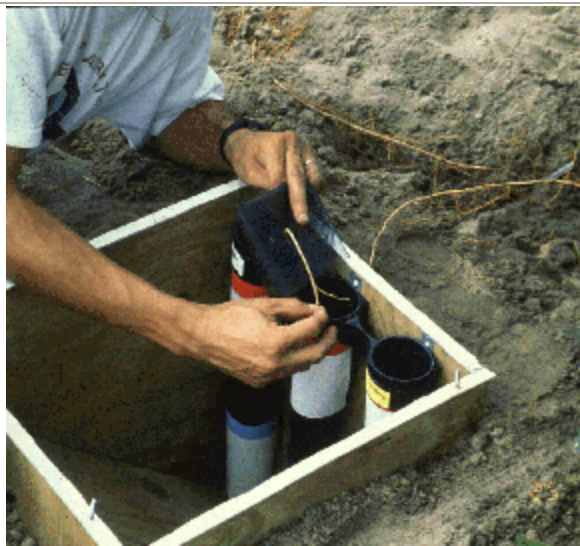
Javier inserting citrus roots of Red grapefruit trees into double-pot system in a root box
