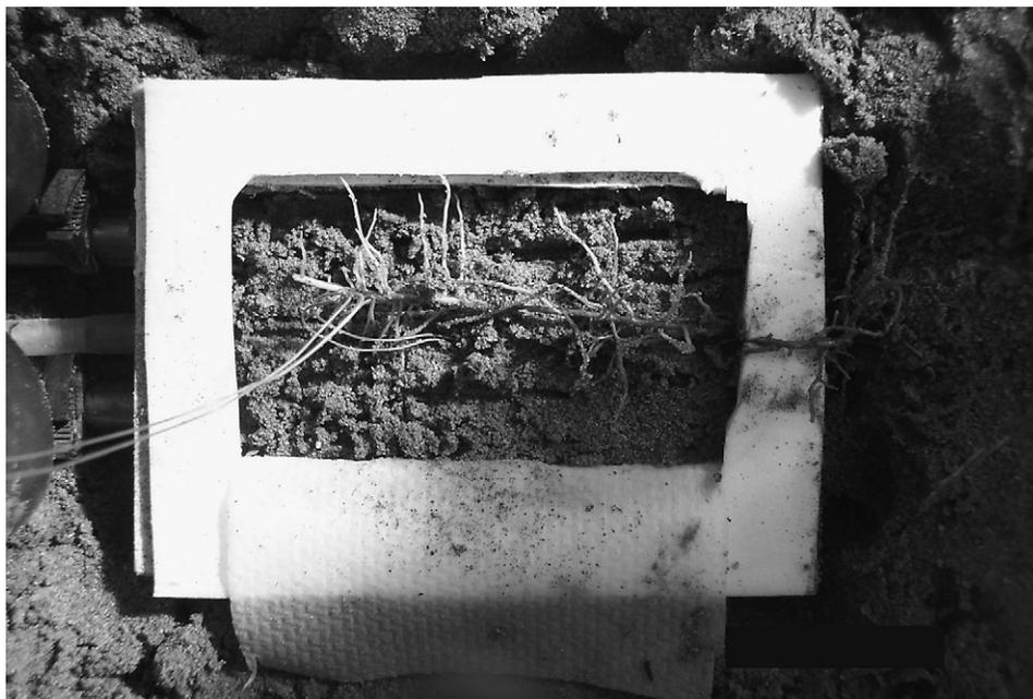
**Fig. 2.** Illustration of Concord grape roots being put in the respiration chamber. The wires are a fine-wire thermocouple.
