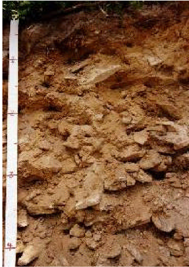
Fig. 12. Typical Hazleton soil profile in a wooded area with the following characteristics: Surface: 0 to 2 inches, dark brown stony sandy loam, Subsurface: 2 to 8 inches, dark gray stony sandy loam, Subsoil: 8 to 10 inches, dark reddish brown channery sandy loam, 10 to 30 inches, yellowish brown very channery sandy loam, Substratum: 20 to 60 inches, light yellowish brown very stony sandy loam, Bedrock: 60+ inches, level bedded gray sandstone.
