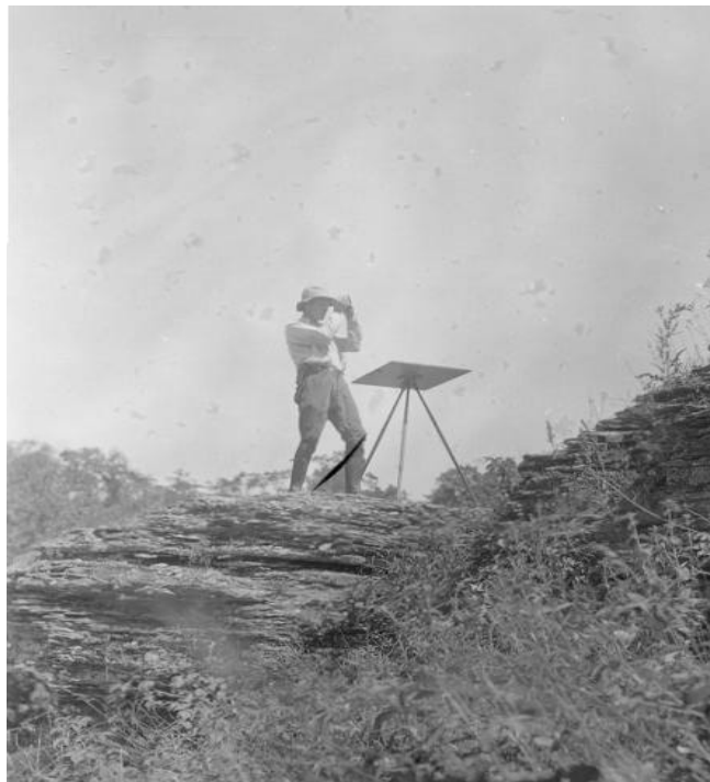
Fig. 9. This photo shows Richard (Dick) Long using a plane table to make a soil map. He is using an abney level to measure slope. The photo was taken about four miles northeast of State College in May 1934.
