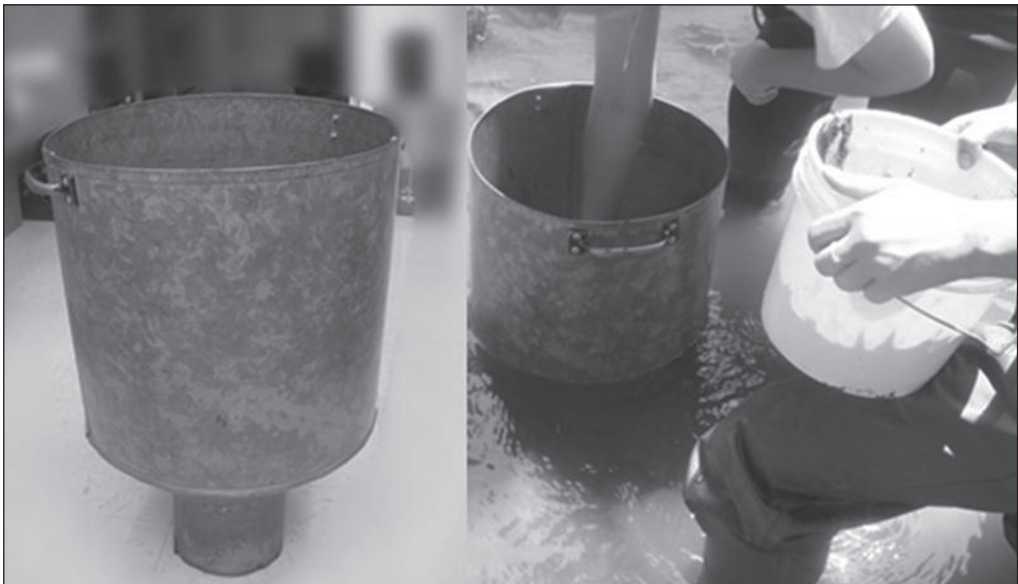
Figure 2. Substrate sampler. Height = 60 cm, neck length = 12 cm, diameter of the upper portion = 36 cm, and diameter of the lower portion = 15 cm.
