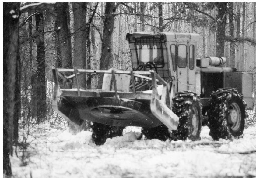
Figure 3. Hydro-axe used to treat areas with a dense understory in order to enhance regeneration of aspen at the Barrens grouse habitat study area.
