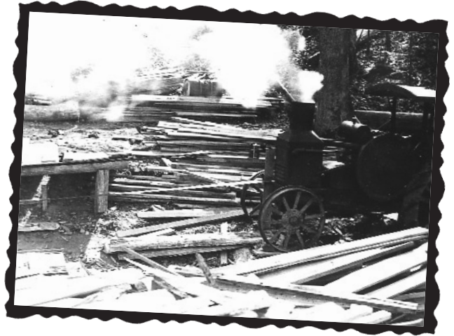
A portable sawmill cuts chestnut logs in Depression-era Shenandoah National Park, Virginia. Courtesy Shenandoah National Park Archives.
